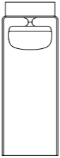
C5 Ceiling Rose Ø 160 mm H 50 mm Diffuser Ø 180 mm H 450 mm
