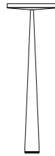
F33 DOWNLIGHT H 2020 mm Diffuser Ø 680 mm H 80 mm Base Ø 200 mm
