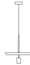
S50 Ceiling Rose Ø 120 mm Cable 3000 mm Diffuser Ø 450 mm H 465 mm
