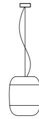
S5 Ceiling Rose Ø 120 mm Ceiling Rose LED Ø 160 mm Ceiling Rose LED DIMM Ø 200 mm Cable 2000 mm Diffuser Ø 360 mm H 450 mm
