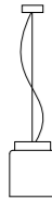
S3 Ceiling Rose Ø 120 mm Cable 2000 mm Diffuser Ø 270 mm H 320 mm
