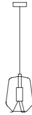
S3 Ceiling Rose Ø 160 mm Ceiling Rose LED DIMM Ø 200 mm Cable 3000 mm Diffuser Ø 320 mm H 450 mm
