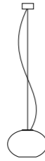
S3 Ceiling Rose Ø 80 mm Ceiling Rose LED Ø 160 mm H 45 mm Ceiling Rose LED DIMM Ø 200 mm H 45 mm Cable 2000 mm Diffuser Ø 280 mm H 180 mm
