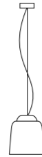
S3 Ceiling Rose Ø 120 mm Cable 2000 mm Diffuser Ø 300 mm H 330 mm
