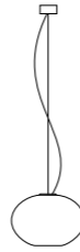
S5 Ceiling Rose Ø 80 mm Ceiling Rose LED Ø 160 mm H 45 mm Ceiling Rose LED DIMM Ø 200 mm H 45 mm Cable 2000 mm Diffuser Ø 350 mm H 240 mm
