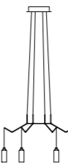
BT6 Ceiling Rose Ø 210 mm Cable 700-1200 mm Diffuser Ø 50 mm H 120 mm
