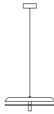
S5 Ceiling Rose Ø 120 mm Cable 3000 mm Diffuser Ø 450 mm H 130 mm
