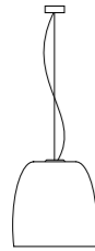
S7 Ceiling Rose Ø 120 mm Ceiling Rose LED Ø 160 mm H 45 mm Ceiling Rose LED DIMM Ø 200 mm H 45 mm Cable 3000 mm Diffuser Ø 480 mm H 490 mm
