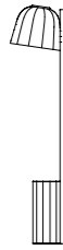
T1 USB H 600 mm Diffuser Ø 130 mm H 110 mm Base Ø 80 mm
