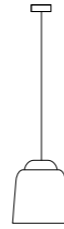
S5 Ceiling Rose Ø 120 mm Cable 3000 mm Diffuser Ø 360 mm H 400 mm
