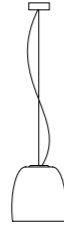
S3 Ceiling Rose Ø 120 mm Ceiling Rose LED Ø 160 mm H 45 mm Ceiling Rose LED DIMM Ø 200 mm H 45 mm Cable 2000 mm Diffuser Ø 300 mm H 305 mm
