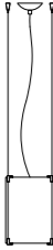
S1 Ceiling Rose Ø 120 mm Cable 2000 mm Diffuser Ø 240 mm H 330 mm
