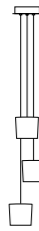
3R - 3S Ceiling Rose Ø 180 mm H 40 mm Cable 3000 mm Diffuser Ø 135 mm H 150 mm
